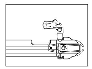
Open the handle of the quick release so the black handle is straight and the fixed end points down. Load the fork onto the quick release so both fork ends are resting straight on the quick release.
