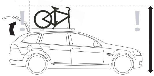
Note the height of your vehicle (including bike) and record it on the sticker provided. Install on the inside of the drivers side sun visor.
