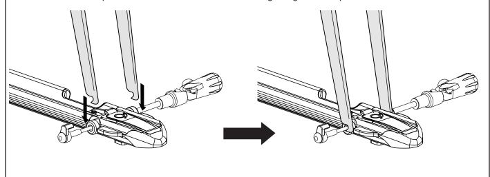
Twist handle clockwise to tighten the quick release skewer. Close the handle by flipping it 90 degrees to the closed position. If it is too loose, open the handle and turn it like a screwdriver (clockwise to tighten, counter clockwise to loosen), and close the handle again. Re-adjust until a firm and positive snap is felt when closed. If locks have been purchased or provided, the cover can now be locked.
