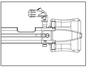
6 Open the handle of the quick release so the black handle is straight and the fixed end points down. Load the fork onto the quick release so both fork ends are resting straight on the quick release.
