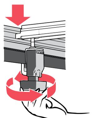
Swing the clamp vertically and align the clamp jaw under the metal truck bed flange. Tighten the T-handle by hand. Do not use a wrench.
