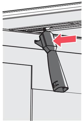
Pull the clamp down and swing it under the truck bed rail edge.
