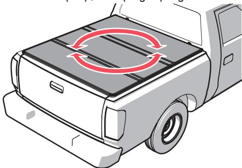
Carefully refold the cover without shifting its position on the truck bed.
