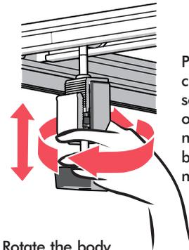
Rotate the body of the clamp up or down to match its position with the bed rail flange.
