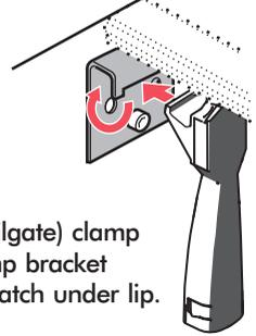
4. Slide rear (tailgate) clamp out to rear clamp bracket pull down and latch under lip.
