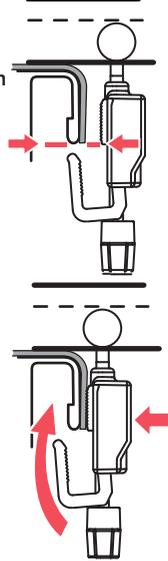
**!** To aid in better water management and the straight appearance of the cover, push down on the cover to compress the seals while tightening the clamps.
