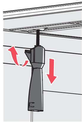
The spring loaded clamp will lock under the truck bed rail edge.
