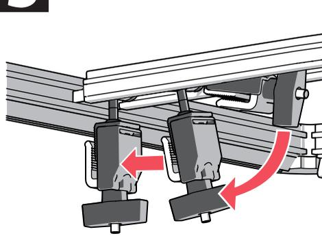
The front (cab) clamp stows in the cover rail. Rotate the clamp down and slide it towards the bed rail.
