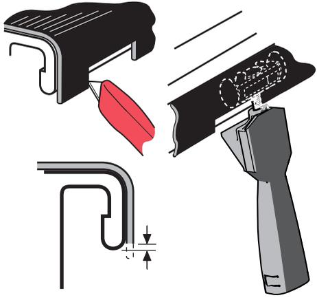
For bed liners that cover the metal flange, trim a minimum of 100 mm or 4" of the liner wall so the clamps contact the bottom of the metal flange.
