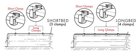
Some trucks use different sizes of clamps to fit curved sidewalls. Longer clamps go in the forwardmost (Cab) positions while the shorter clamps hold the rails at the rear (tailgate) end.
