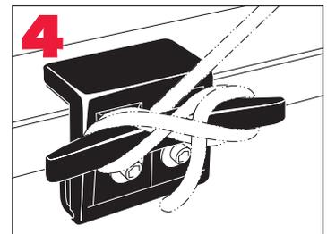
All weight bearing rope or hooks MUST be in the CENTER hole as shown below.
