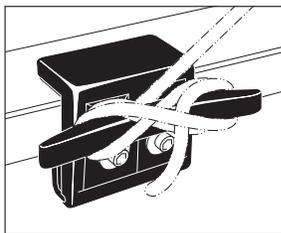
**IMPORTANT:** All weight bearing rope or hooks MUST be in the CENTER hole as shown above and as shown in the tying diagram below.
