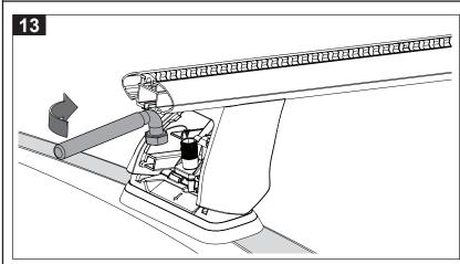
Locate M6 screw into stud. Tighten plastic bolt housing alternately both sides.
