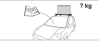
When these roof racks are to be used on a vehicle that is driven off sealed roads, the manufacturer maximum roof load rating (to be found in the vehicles User Manual) should be *halved*. Do not forget to subtract 5kg from your maximum carrying capacity due to the weight of the crossbars and legs.
