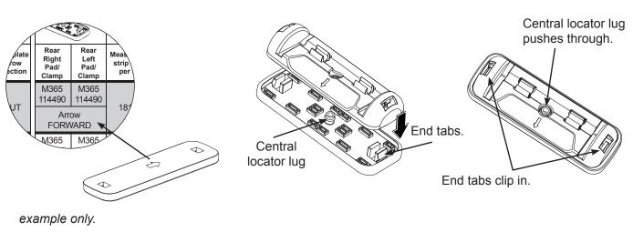
Clip foot plate onto base of the leg with the arrow facing In or Out according to your vehicle listed in the DK specification sheet.
