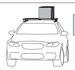
70kg load rating (Urban road) = 35 kg load rating (Off road - 70kg / 2)
