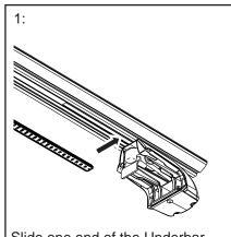
Slide one end of the Underbar strip in behind the Leg as shown.
