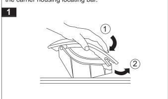
Below are the 2 positions in which the carriers can be fitted to suit various kayak / canoe shapes. When using the tie down straps provided please fasten as shown below. After securing the kayak or canoe, check the load for safety.
