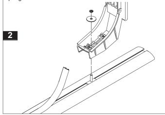
Screw the M6 wing nut onto the T-bolt with 2 turns.
