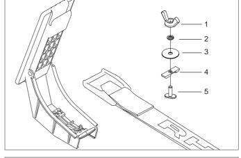
**RHINO** bars: Insert the M6 T-bolt into the top recess of the cross bar and turn 90 degrees. Assemble the T-bolt tab onto the T-bolt, ensuring that the T-bolt tab locks over the T-bolt flange. The T-bolt tab must be level or below the top surface of the crossbar when assembled.
