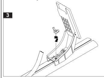
Adjust the carriers to suit the kayak or canoe. Tighten the wing nut to secure the carrier. Cut the rubber buffer strip to suit.
