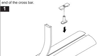
Place the carrier onto the M6 T-bolt through the center mounting hole (front or rear hole). Assemble the flat and spring washers onto the T-bolt.
