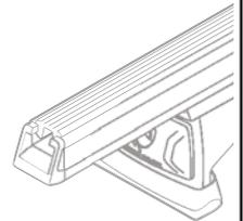
**1** Place the base pads on the roof rail at 290mm from the front join on the roof rail then 605mm between the pads. Install crossbars as per corresponding instructions.
