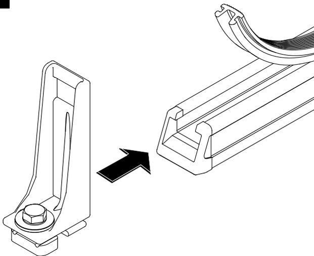
Position the load holder, turn the attachment bolt so that the channel nut rotates and locates across the crossbar, tighten. Trim rubber buffer strip to suit.
