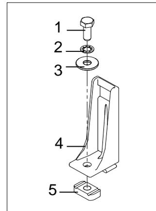
Remove the rubber buffer strip from the crossbar. Loosen the channel nut and slide the load holder T shaped section into the top recess of the Rhino crossbar.
