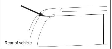
Set the legs in the position shown below when using 3 crossbars. The rear leg sits up against the rear piece of gutter trim. Rear legs use 1 leg height spacer per leg to make all 3 bars level.
