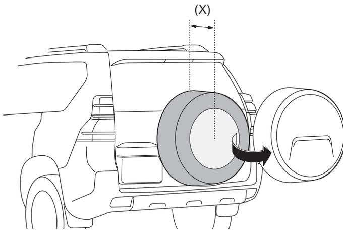
**2** Loosen the Carrier Arms by turning the Locking Knobs as shown. Lift the Arms to a **90 degree angle** and tighten in place. Do not over tighten as adjustments may be needed later.
