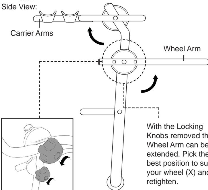
With the Locking Knobs removed the Wheel Arm can be extended. Pick the best position to suit your wheel (X) and retighten.
