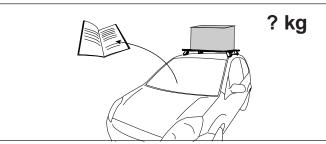
When these roof racks are to be used on a vehicle that is driven off sealed roads, the manufacturer maximum roof load rating (to be found in the vehicles User Manual) should be *halved*. Do not forget to subtract 5kg from your maximum carrying capacity due to the weight of the crossbars and legs.
