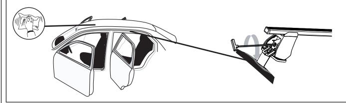
Insert the two lugs on the side of the front cover into the leg, using the key provided turn the lock barrel to the open position (O), engage the locking tab into the leg and turn to lock. Refer instruction 14 below for lock positions.
