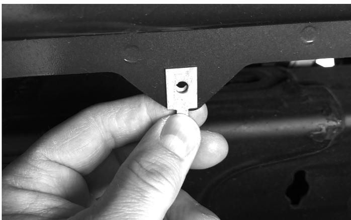
4. If your truck was not equipped with factory wheel well liners install a u-clip at locations B, C, and D by clipping the u-clip over the tab and aligning with the factory hole.
