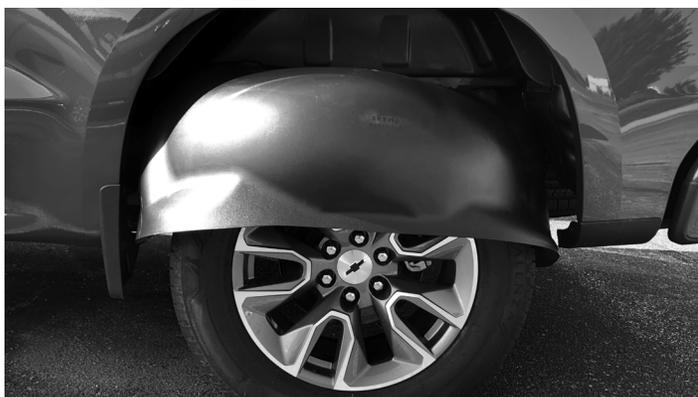
5. Insert the Wheel Well Guard into the rear wheel well opening over the tire.
