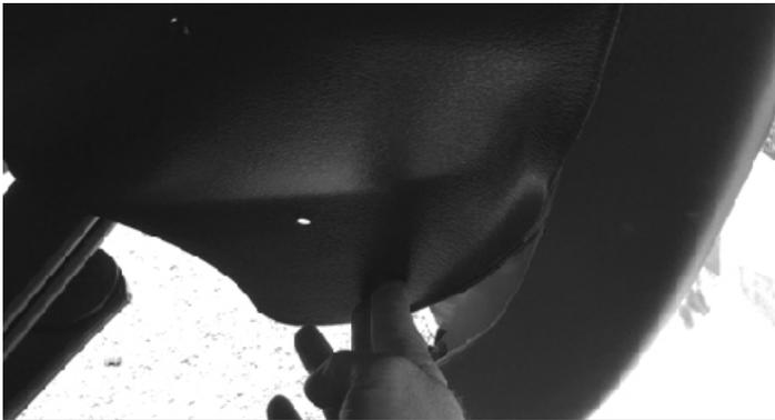
7. Tuck the Wheel Well Guard behind the fender lip starting at the rear of the vehicle first and continuing all the way around the fenderwell opening.
