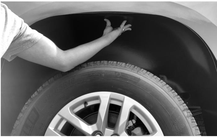
6. Push The Wheel Well Guard up into the wheel well opening.
