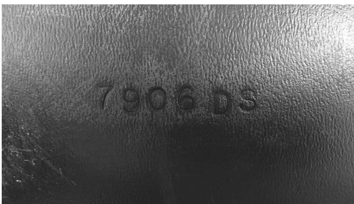
3. Verify that you are installing the correct Wheel Well Guard by checking the part no. located on the backside of the part.
