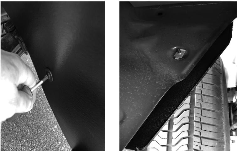
9. Align the 5 holes in the Wheel Well Guard with the factory screw locations and install the factory torx head screws. Install all screws before tightening.
